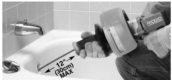
Figure 8 – Move Hand Grip Toward Drum To Grip Cable With Chuck
