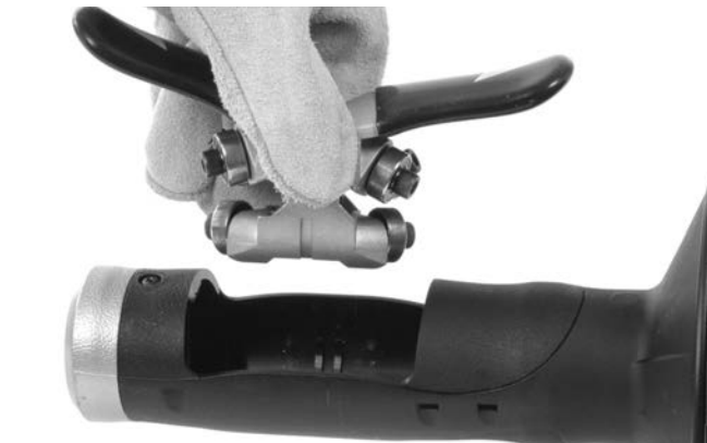
Figure 12B – Removing AUTOFEED Mechanism From Housing
