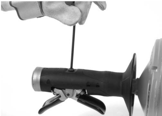
Figure 12A – Removing AUTOFEED Screw
