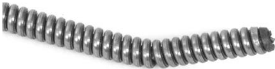
Figure 15 – Bend At Cable End
