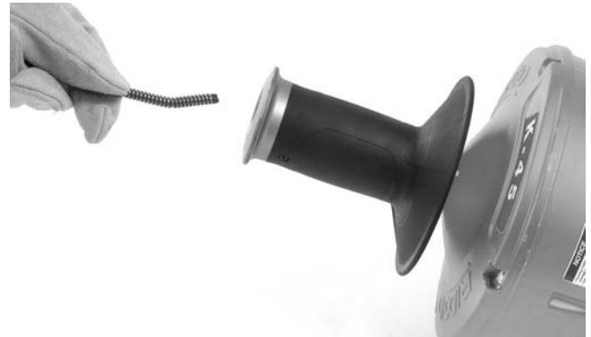
Figure 17 – Loading Cable Without Changing Inner Drum
